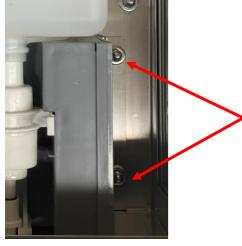
**Step 1:** Loosen the left and right fixing nuts.
